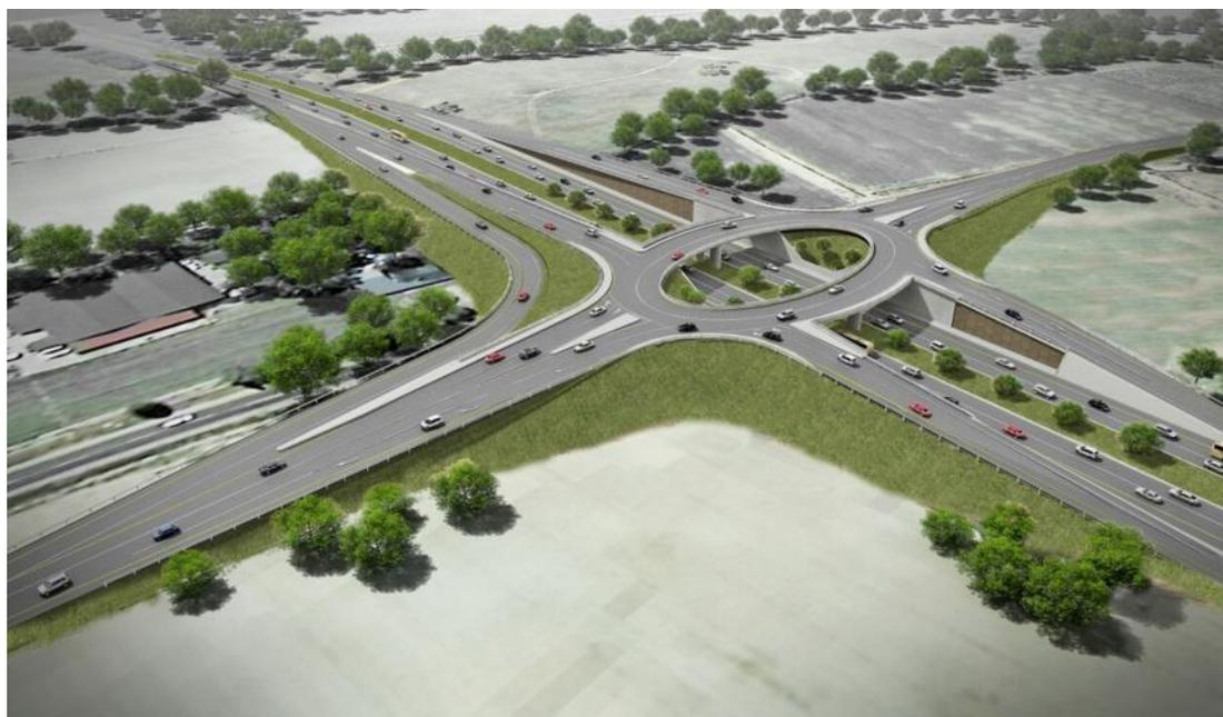
**Figure 4. Aerial perspective of proposed roundabout interchange**
